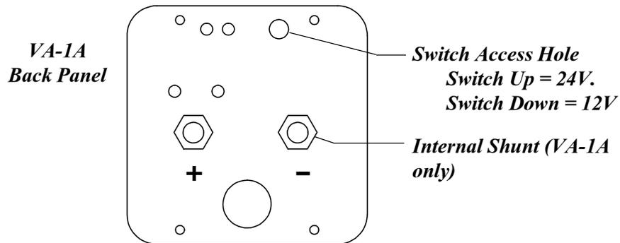
3. Determine how the VA Unit will be installed in your aircraft’s electrical system:
