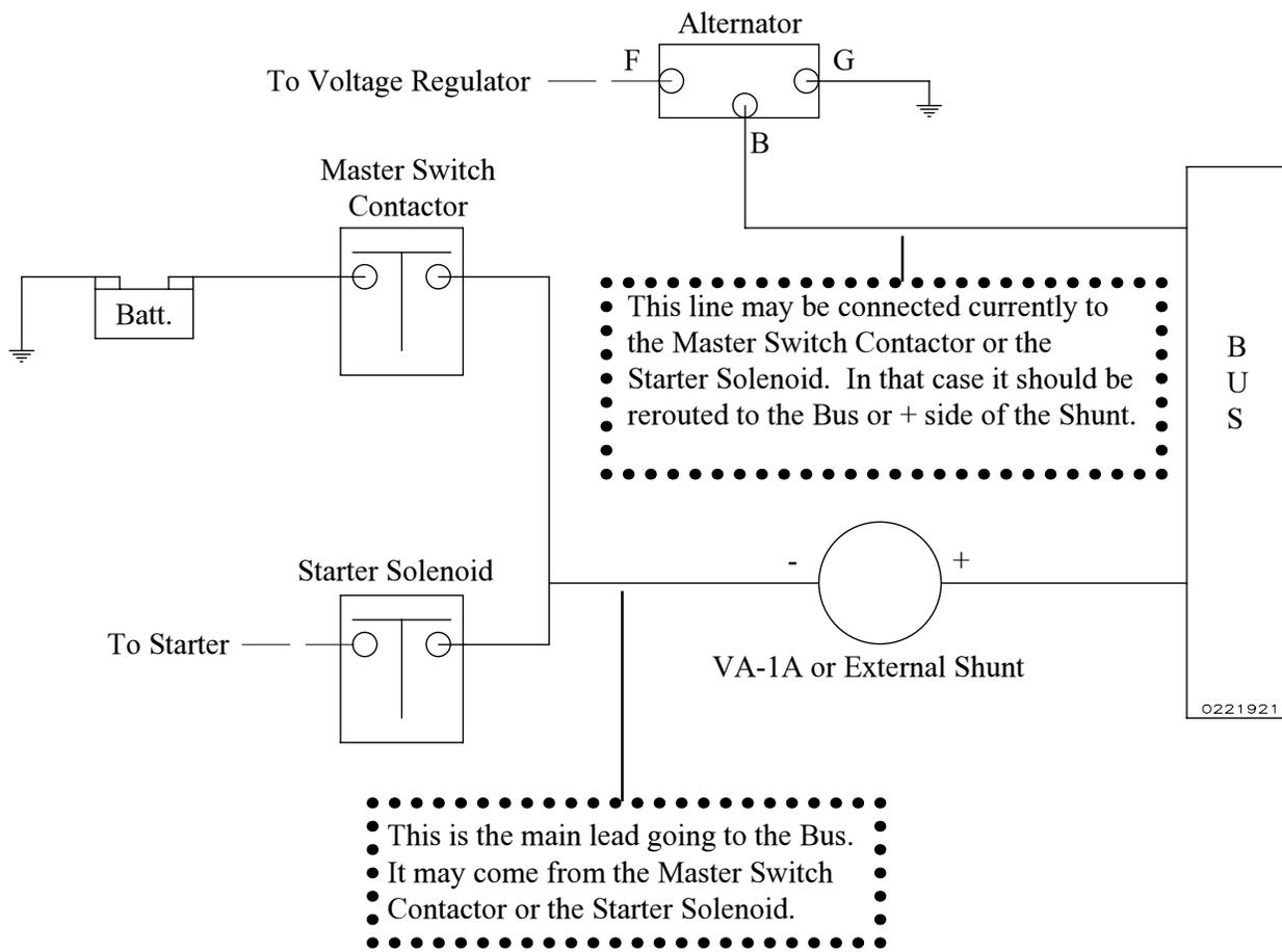
Note: The VA-1A or External Shunt should not be installed in series with the starting current.
