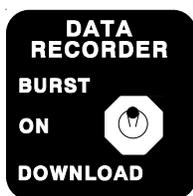
If the Control Switch is placed in the "ON" position, the Data Recorder will store data to internal memory according to the Storage Time Interval setting (1, 3, or 6 minutes) set by the DIP switches found in an opening on the side of the Data Recorder's black box.
