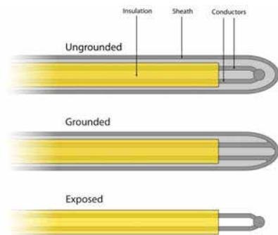
Most of Electronics International's probes are ungrounded and are not effected by ground loops, noise or voltage shifts. In addition, Electronics International incorporates common mode amps, differential inputs and filters to insure accurate and stable temperature readings for grounded probes.
