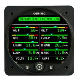
The CGR-30P and CGR-30C systems are identical in hardware, installation and maintenance. The difference between the two models is the configuration of the user screens. The CGR-30P incorporates two arcs at the top of the display, a bargraph display for monitoring EGTs & CHTs and strip gages for other functions. The CGR-30C only displays strip gages.
